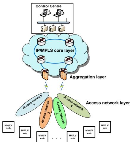
Figure 2: The three level hierarchy of the Elektro Primorska communication network
