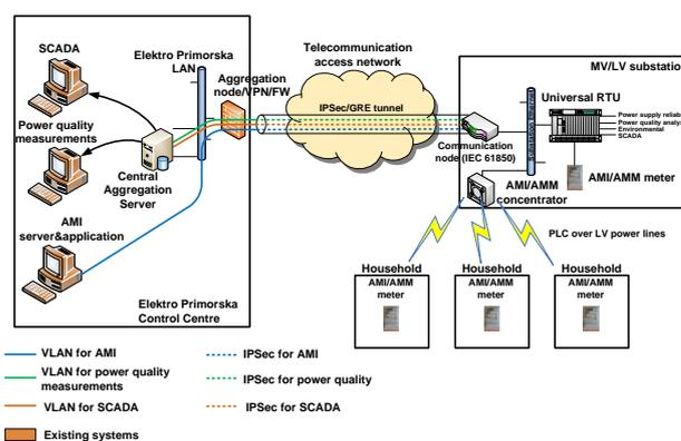
Figure 1: The concept of the integrated MV/LV substation integration through unified telecommunication network
