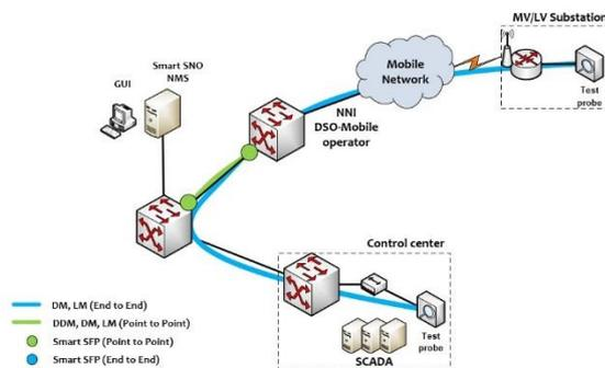
Figure 5: Mobile network used as alternative for MV/LV substation integration with Ethernet optical segment in DSO's ICT network
