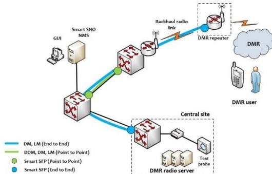
Figure 4: DMR radio system integrated with Ethernet optical segment in DSO's ICT network
