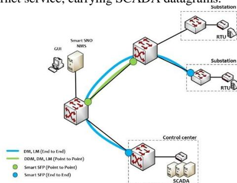
Figure 3: Ethernet optical segment in DSO's ICT network
