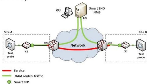
Figure 1: Typical integration of OAM functionalities into ICT network
