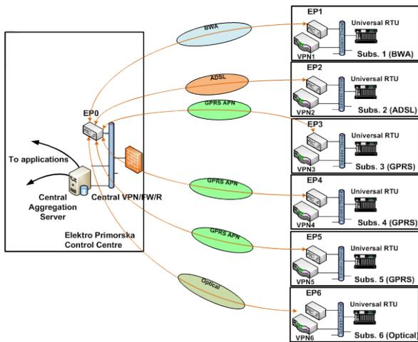
Figure 3: The topology of throughput tests at Elektro Primorska
