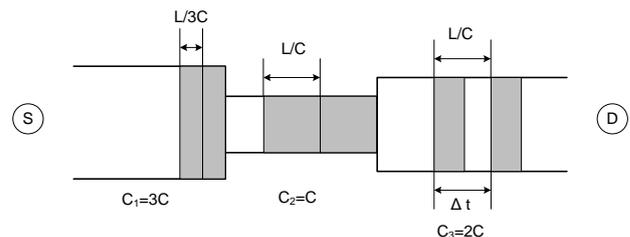
Figure 2: Technique of packet pairs for capacity test
