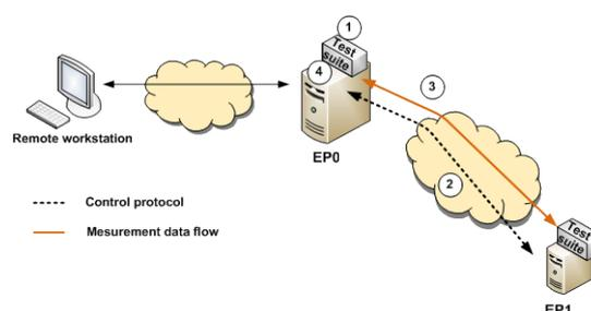
Figure 1: The principle of the throughput tests
